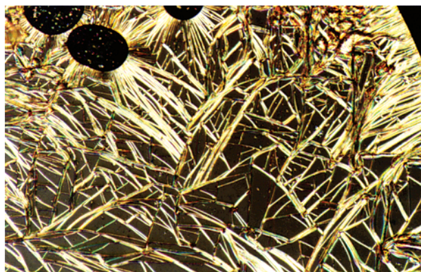
Figure 1. Polarized optical microscopic texture of the TGBA* phase of 1a on heating from homeotropic SmA texture (113.8 °C).
